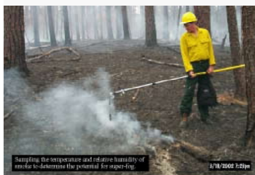
Figure 2. Sampling temperature and relative humidity of smoke from smoldering logs in the wake of a prescribed burn in central Georgia.
