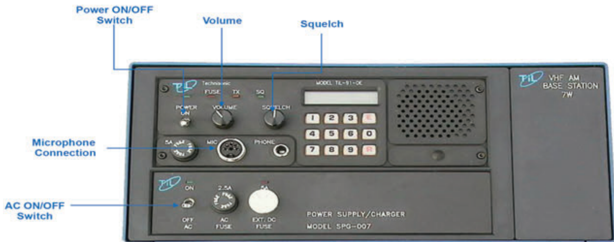
Figure 2: TBS-150 Base Station (Located in building or Tent)
