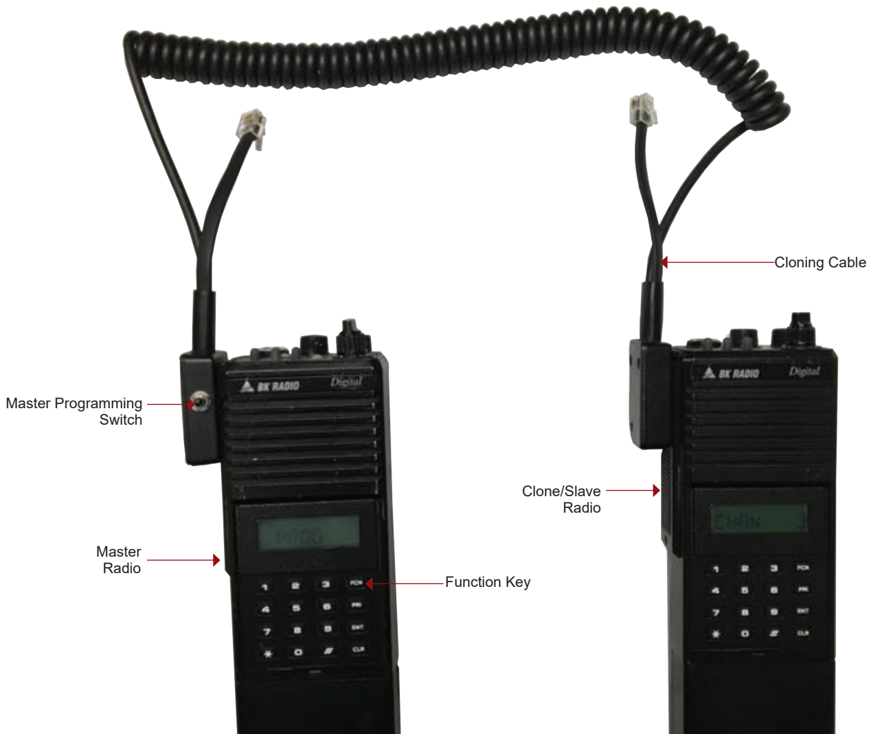
DPHx Cloning Connections
